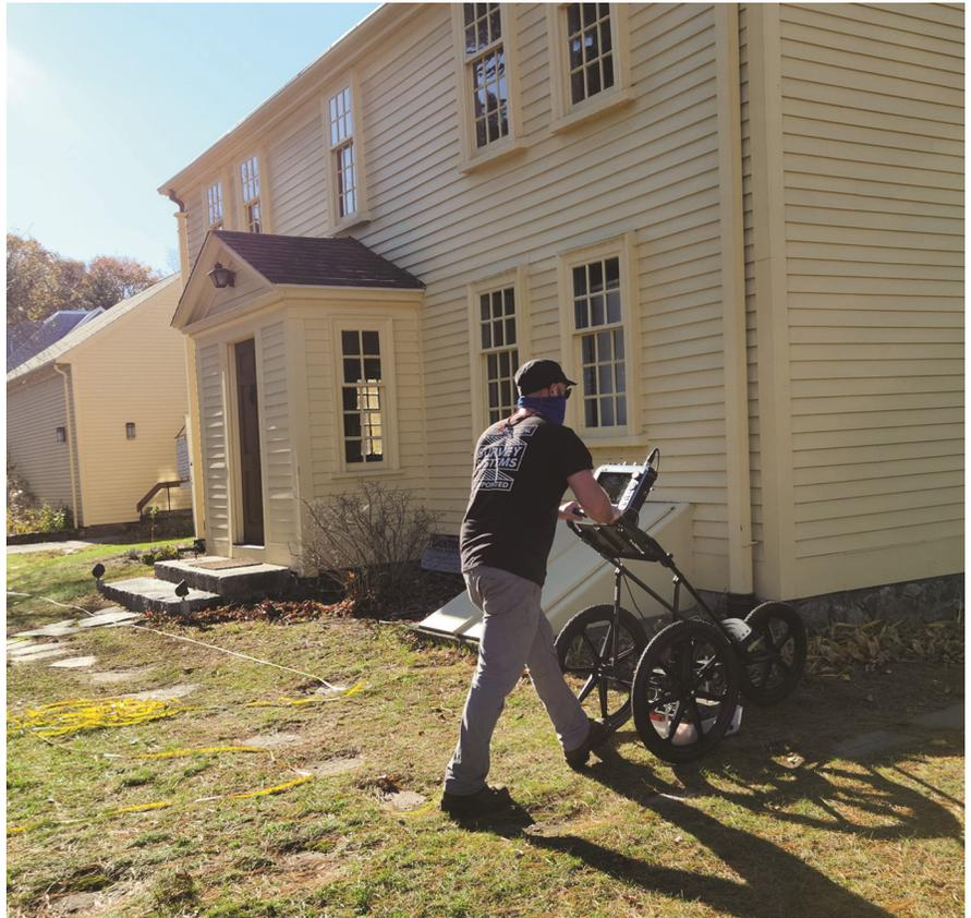
Geophysical Survey Systems, Inc., conducted ground-penetrating radar investigation of the Jason Russell House grounds on November 10, 2020. The remarkable technology will help to understand what is below the ground without disturbing it. GSSI also did this work pro bono as their way to give back to the community. It sounds as if they found a few interesting things, but we will have to wait for their report to find out.
